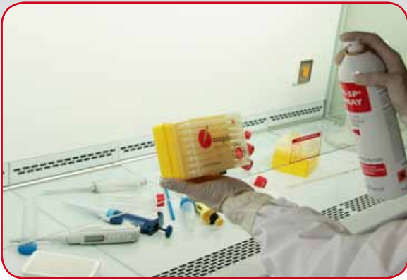
7. Wipe all material with sterile 70% alcohol before transfer it inside the bench and before to start the activity
