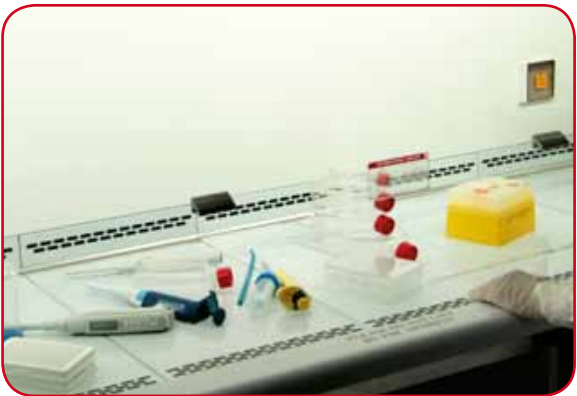
13. Three separate areas inside the working bench: right "clean", centre "working", left "dirty"
