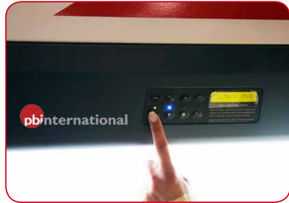
2. Switch on the BSC / UAC five / fifteen minutes before to start the activity
