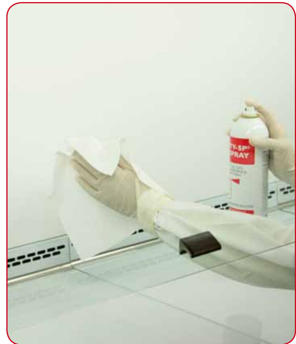
16. Clean and disinfect all the surface of the inside BSC at the end of activity
